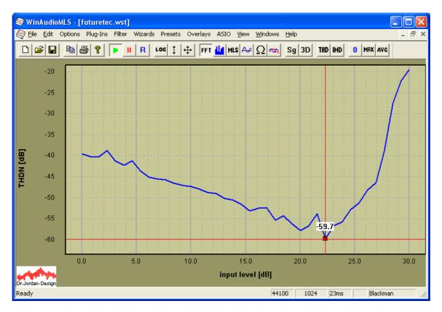
The distortion drops until a minimum at 22.2dB=166Watt to -59.7dB (0.1%)
