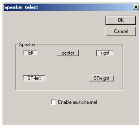
The signal generator supports up to 5 output channels. You can disable this feature to run on stereo soundcards. From a selection matrix you can disable or enable all speakers.
