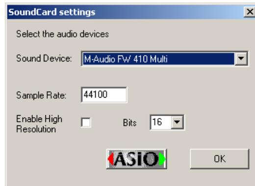
The signal generator supports multiple soundcards in your PC. Select the desired soundcard from the selection box. You can also adjust the sample rate. If you enter a value, which is not supported by your hardware you get an error message or no signal output. This behavior depends on the soundcard driver. Typical sample rates are 32000, 44100 and 48000Hz.
