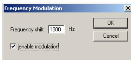
With the FM-modulator you can generate many different signal types. The following example shows how to generate a signal that switches every second between 500Hz and 1000Hz. First we need a rectangular signal with a frequency of 0.5Hz. With a DC offset of 2.0, we shift the signal to a level range of 1.0 to 2.0. In FM-mode there occurs no overdrive, because the DC offset is handled in a special way. The frequency shift has to be set to 500Hz.
