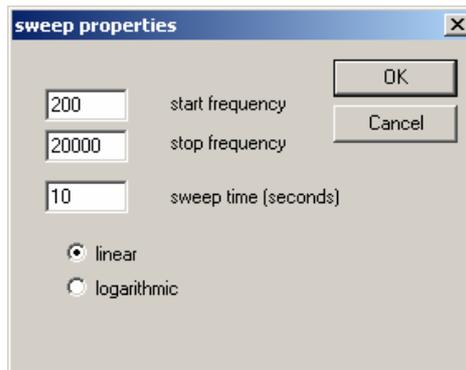
You can also choose between a linear and logarithmic sweep. A linear sweep increases the frequency by a constant value every second. The logarithmic sweep instead starts slowly and speeds up. This results on a typical logarithmic frequency scale in a constant speed. The sweep time of one octave is constant.
