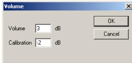
In this dialog box you can also a calibration offset that is applied to all levels.
