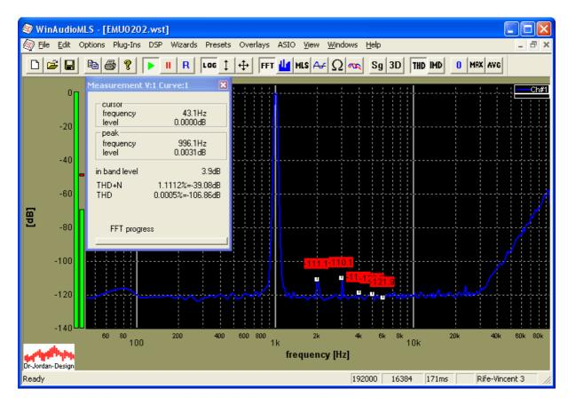
Significant aliasing components above 30kHz which reduces the wide-band THD+N. We can remove such components with a digital low-pass filter.
